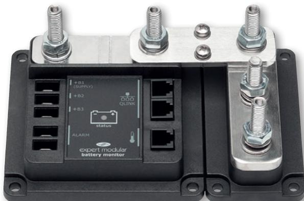
The Expert Modular active shunt base has a Grid Optimized footprint. This enables perfect system integration with busbars and fuseholders from the TBS DC Modular product lineup. The picture on the left shows a nice solution to avoid stacking all battery negative return cables on the single "System side" stud of the shunt.
